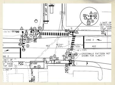
Crosswalks should always be located between the stop line and the intersecting roadway. A problem frequently observed on installations is when a sidewalk is offset from the roadway, a crosswalk is located at the same distance from the intersection. This results in the crosswalk located in advance of the stopping location. The mitigation for this is to move the sidewalk closer to the intersection.
