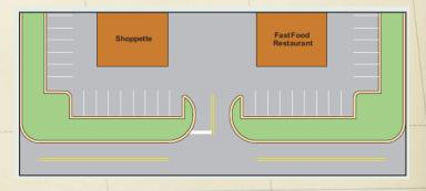
Proper spacing for roadway access points must be considered when designing an intersection. The recommended spacing varies based on speeds and roadway type. The following table shows the recommended access spacing.
