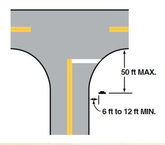
The stop line location is related to the crosswalk and accommodating truck turning movements. If a truck is the design vehicle, it should be able to turn through an intersection without conflicting with stopped vehicles on other approaches. Specifically, the stop line should be far enough back to avoid a truck turning path. The location where the stop line must be placed to avoid a turning vehicle's path is also the location of the Stop sign.
